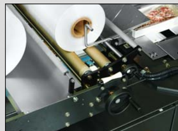
EZ Load film Cradle with Flip Away Guides & Hand Wheel Adjusters, Film Loads & Adjusts From Both Sides of Wrapper
